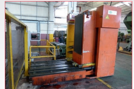
• Herwo 13-Ton Capacity Electric Die Loader (1999)
