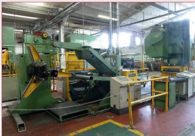
• Rhodes 400-Ton Double Sided Press with Atkin Decoiler, Leveller, Servo Feed Unit & Scrap Conveyor, Bed Size: 60" x 48", Adjustable Stroke: 2" - 8"
