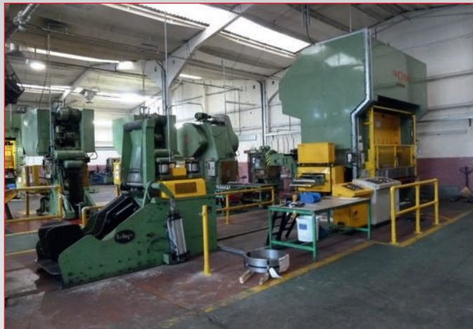
• Rhodes S2-400-108/60 400-Ton Double Sided Press with BHP Decoiler, Leveller, Atkin Servo Feed Unit & Scrap Conveyor, Bed Size: 108" x 60", Shut Height: 12" - 24"
