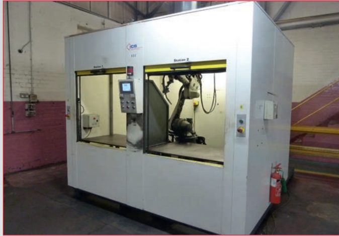
• 8 x Panasonic Twin Station Robotic Mig Welding Cells (1998-2010)
