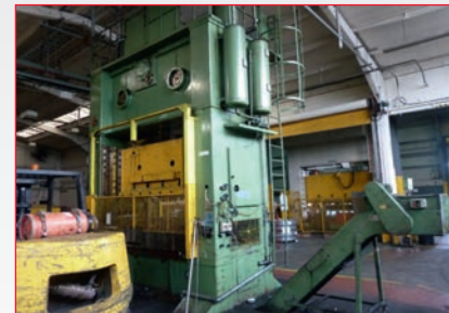
• Stanko 315-Ton Double Sided Press with Clark Decoiler, Atkins Leveller, Servo Roll Feed & Scrap Conveyor, Bed Size: 2500mm x 12500mm
