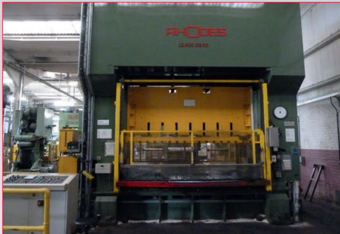
• Rhodes S2-400-108/60 400-Ton Double Sided Press with BHP Decoiler, Leveller, Atkin Servo Feed Unit & Scrap Conveyor, Bed Size: 108" x 60", Shut Height: 12" - 24"
