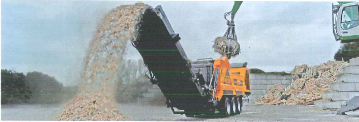
Grinding of waste wood/pallets
