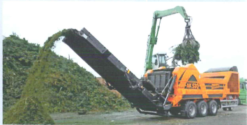
Grinding green waste
