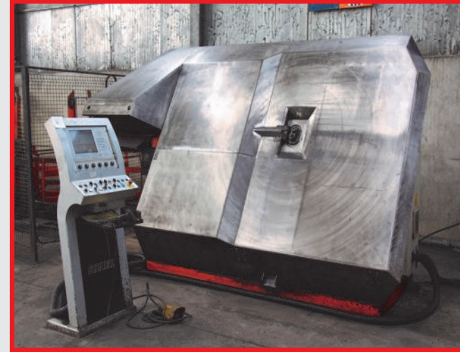
Schnell Formula 12 HS VG Dual Directional Stirrup Bending Machine (2003)
