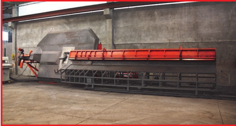
Schnell Coil 18 BE EL Dual Directional Stirrup Bending Machine (1997)
