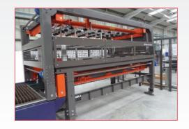
ABB R300 Single LC Robotised Welding Cell with ABB 6-Axis Welding Robot, Fronius Welding System & IRBP R-300 Twin Sided Welding Positioner (2011)
