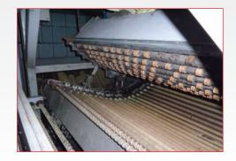
• **Glamec** Tempering Furnace Type RHF 158/220-3.0/19-L-ECE with Preheat Furnace (1990)
