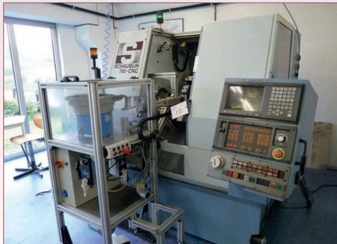
• Schaublin 110-CNC Slant Bed CNC Lathe with Fanuc 18T Control, Tumac Bowl Feeder & Loader, Platern Tools (1997)
