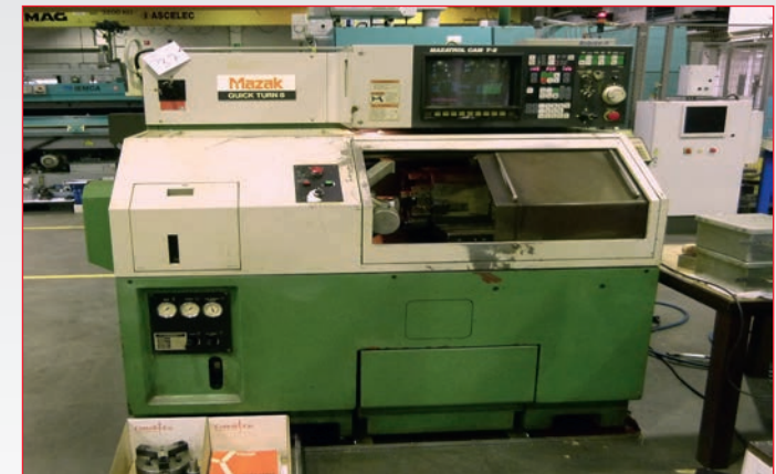
• Mazak Quick Turn 8 CNC Lathe with Mazatrol CAM T-2 Control, Turning Capacity: 160 x 250mm, 8-Station Turret, Collet Chuck, 3-Jaw Chuck, Turret Tools, Tool Presetter & Tailstock
