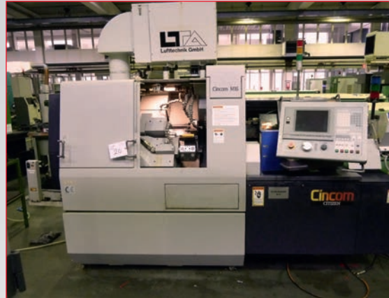
• Citizen Cincom M-16 CNC Sliding Head Lathe with Mitsubishi Meldas Control, 10-Station Turret, Sub-Spindle, Parts Catcher, Parts Conveyor (2000), Lemca Boss 432/32 Magazine Barfeed (2000), Lufftechnik Mist Extraction
