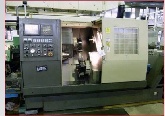
• Hardinge Conquest Twin Turn 65 7-Axis Turning Centre with Fanuc 18iT Control, Twin 12-Station Turrets with Driven Tools, (1998 - USA Built), Swarf Conveyor, Parts Catcher & Conveyor Promatec Mist Extraction, Lemca Tal Auto 65/32 Mag Barfeed (1999)
