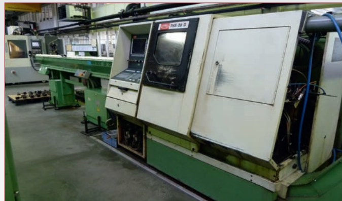
• (2) Traub TNS26DGY Multi Axis CNC Lathes with Traub System TX8F Controls, Sub-spindles, Twin 12-Station Turrets, Driven Tools, Parts Catchers, Parts Conveyors, Swarf Conveyors, Lemca Mini Boss 32 & Traub Stamag DN26 Magazine Barfeeds
